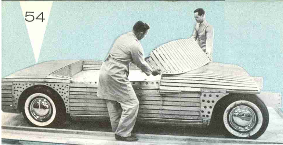
Clay modelers position windshield on wood armature. Slatted construction anchors clay.
