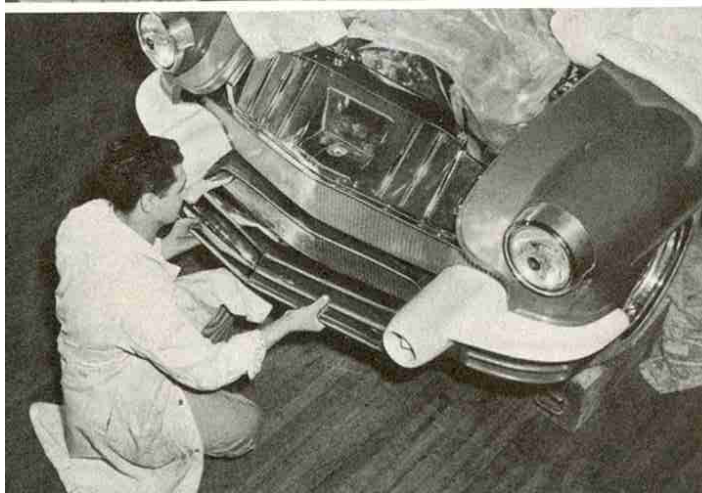
(Above) With the car almost completed, the plastic-coated windshield is fitted in place. Great care must be taken here to insure even pressure in the supporting molding. (At left) Chrome-plated bumper plate is positioned. Temporary white plastic covering protects other bumper parts.
