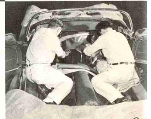
Floor covering is fitted to underbody prior to installation of seats.
