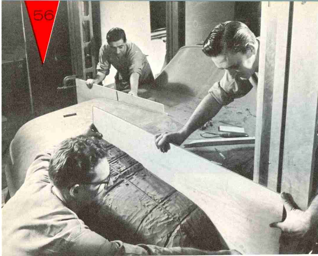
Modelers in foreground work on near side with template taken from and matched to opposite side. The result is two identical sides.
