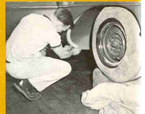
Painter prepares to touch up damaged paint. Note rubber boot on wheel. It will protect tire against damage during shipment.
